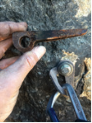
LEFT The old piton in a pocket that protected the crux of Mark’s Moderate came out very easily. Jerry Dodrill removed it and then took liberty to install a bolt at the same height.
